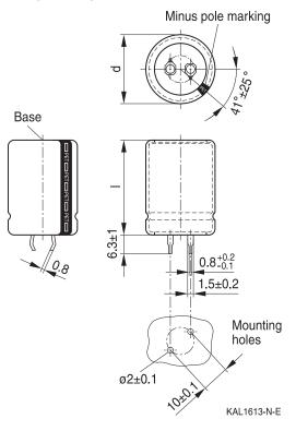
Snap-in terminals, length  $(6.3\pm1)$  mm. Also available in a shorter version with a length of (4.5-1) mm. Insulation is marked with label "PET" on the sleeve. Safety vent on the base.
