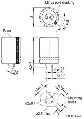
Snap-in capacitors are also available with 3 terminals (length (4.5-1) mm). Insulation is marked with label "PET" on the sleeve. Safety vent on the base.
